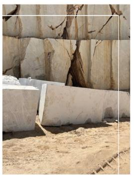
• Azna stone is usually cut in large dimensions, which are called slabs. Azna stone slabs are used for flooring and wall cladding in buildings. This stone achieves an excellent finish when polished. Azna porcelain crystals are small and have a high density.
